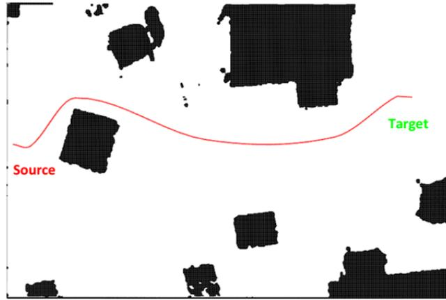
Figure 12: *RRT-PCHIP* smoothed path linking *Source* to *Target* visualized in *RVIZ*.
