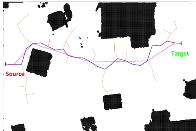
Figure 11: *RRT* planning with a step size of 40 pixels visualized in *RVIZ*.
