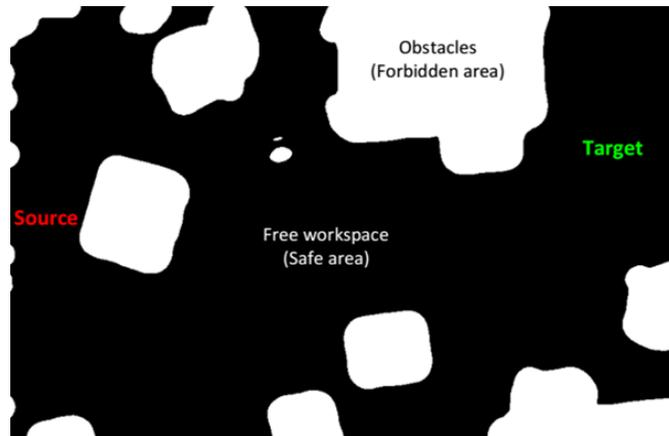
(c) Obtained safe map (Kinect 1 + Kinect 2).
