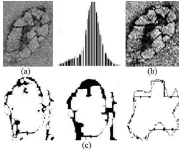
Figure 1: The result of image pre-processing, (a) original image, (b) image after filter step, (c) image of edge detection and morphology step.
