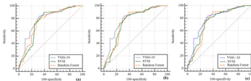
Figure 6: Results of analysis ROC for classification of road defect (a) INESC TEC, Portugal, (b) Irkutsk Russia, (c) Thai Nguyen Viet Nam.
