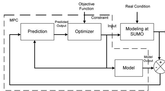
**Figure 4.** Block Diagram of the Traffic Control System
