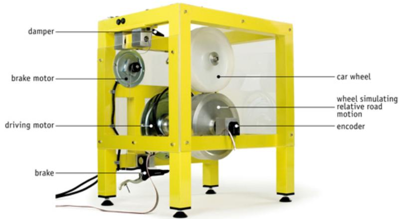
Figure 3: INTECO ABS physical model
