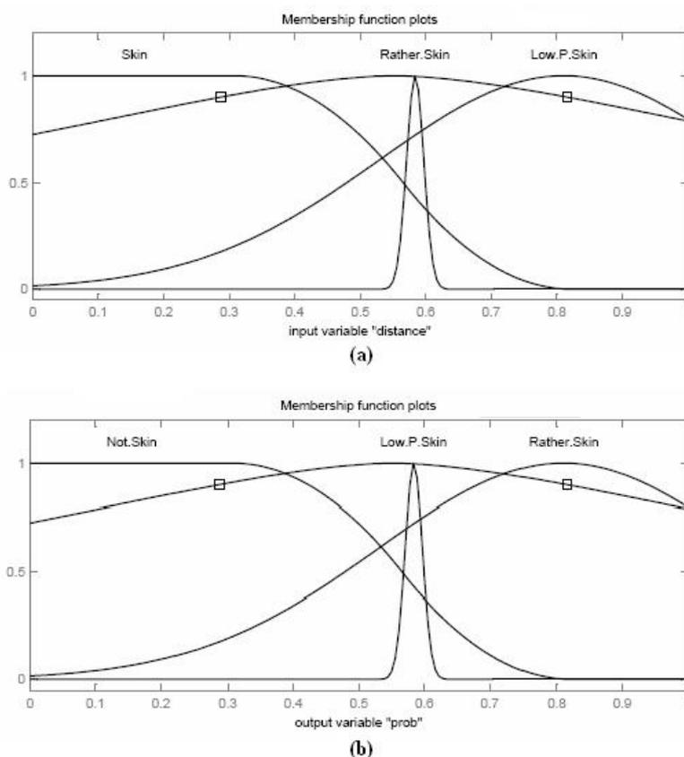
**Figure 1.** a) input MF and (b) output MF of skin color classification system
