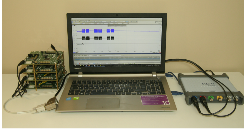
Fig. 5. Experimental FlexRay network setup used for testing proposed attacks
