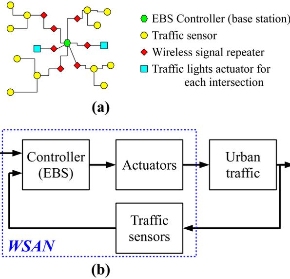
Fig. 4. WSAAN architecture with explicit ensemble-based controller. (a) Network general topology, (b) Abstraction of traffic control application.
