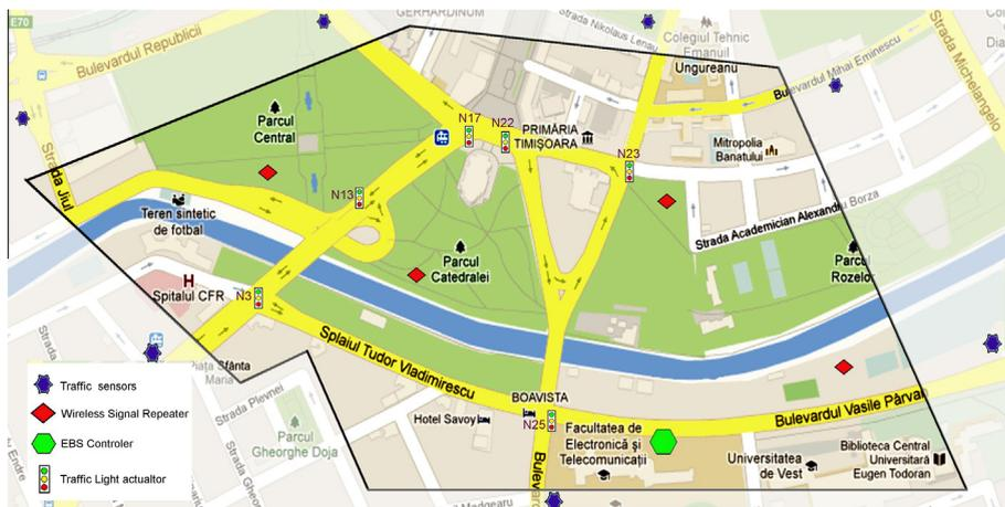
Fig. 5. Investigated area in the center of Timisoara with WSAN deployment.
