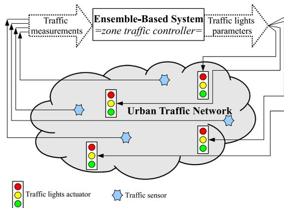
Fig. 2. Ensemble based system as an on-line decision making entity for adaptive traffic lights control.
