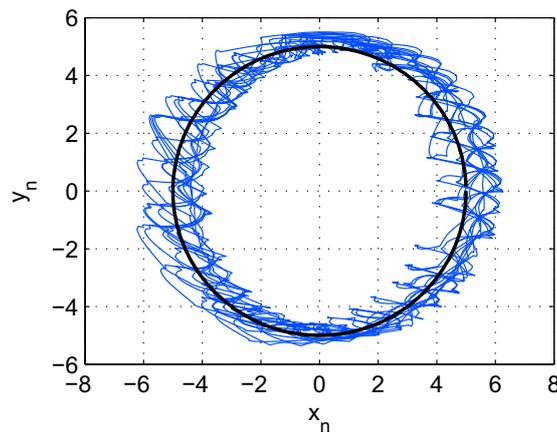
Fig. 6. The circular guiding line and corresponding chaotic path of the differential patrol robot ( $k_1 = 1.5$ ,  $k_2 = 4$ ).
