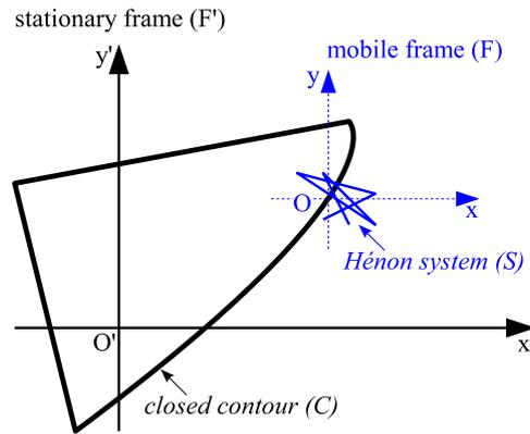
Fig. 3. Obtaining the chaotic path via relative motion.
