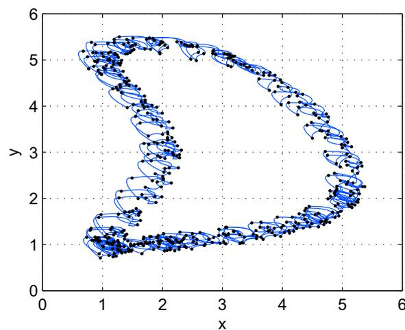
Fig. 12. Chaotic robot path in the proximity of closed curve (two complete laps along the guiding line).
