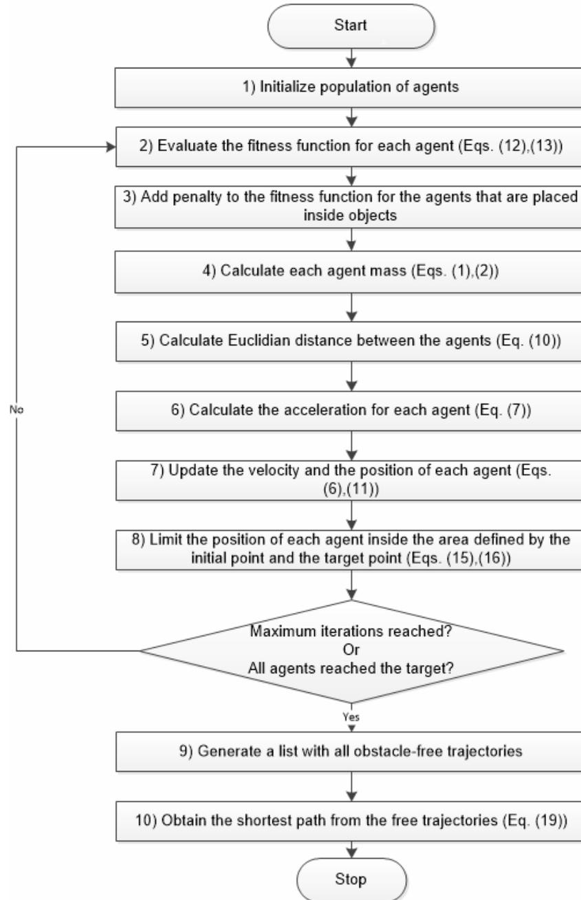
**Figure 1.** Flowchart of the GSA-based off-line algorithm.
