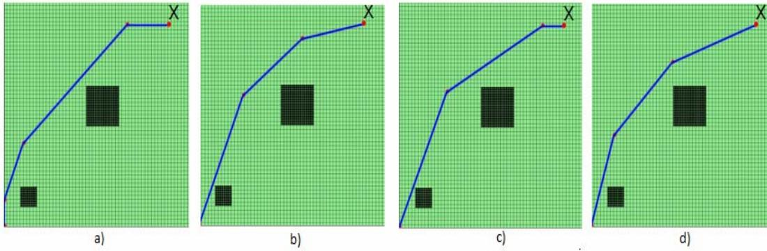
**Figure 5.** PSO-based solutions in a simple environment.
