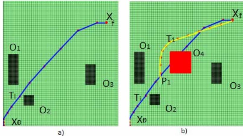
**Figure 11.** On-line path planning in a partially-known environment.
