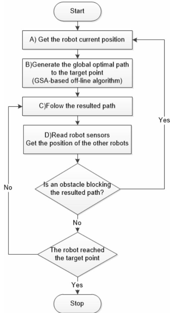
**Figure 3.** Flowchart of on-line path planning algorithm.
