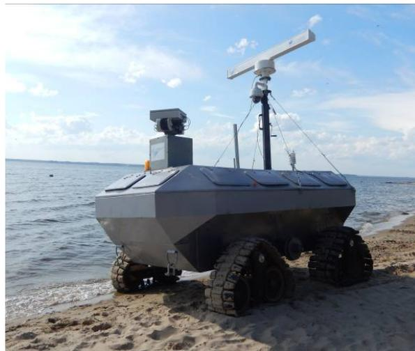
**Figure 2.** The mobile robotic system for coastal zone monitoring: track movers.
