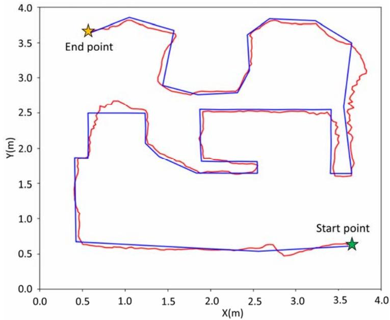
**Figure 17.** The passed ways during the experiment (blue line – planned path during simulation, red line - real execution)
