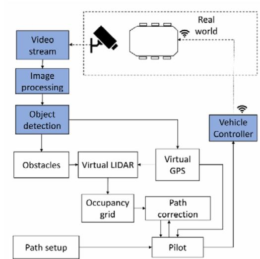
**Figure 4.** The structure of the software for unmanned movement in the laboratory environment.
