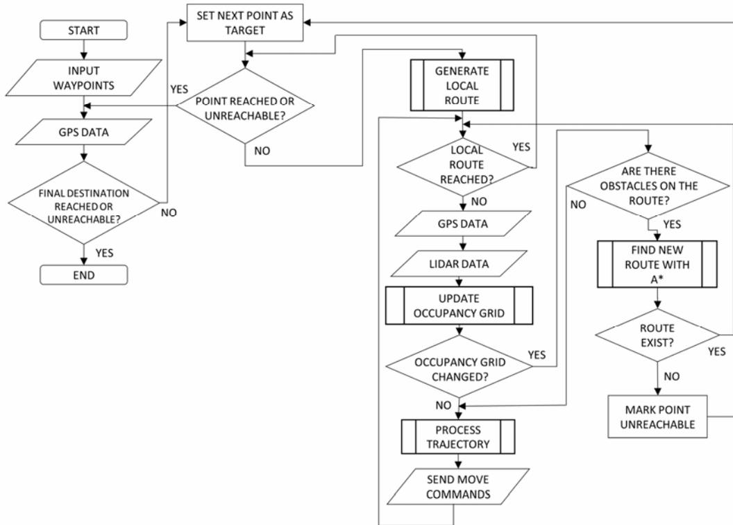
**Figure 5.** The unmanned movement algorithm diagram.
