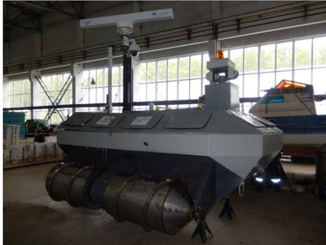
**Figure 3.** The mobile robotic system for coastal zone monitoring: rotary-screw movers.
