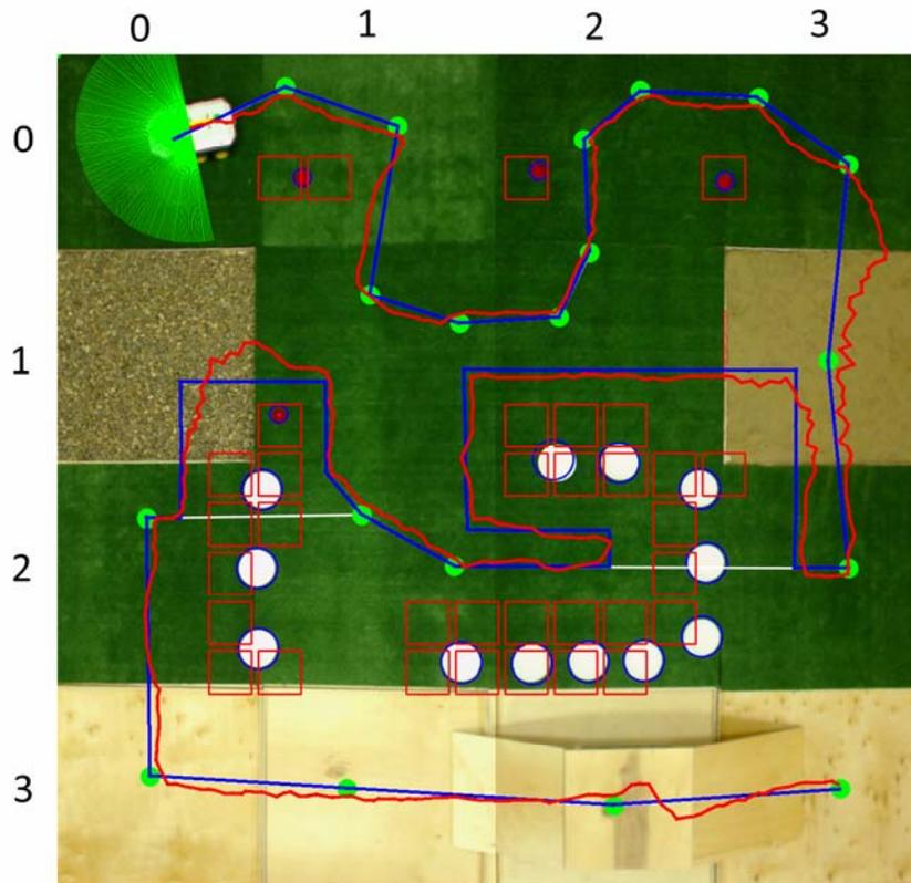
**Figure 16.** Planned (blue line) and passed (red line) ways of the robot during real execution.
