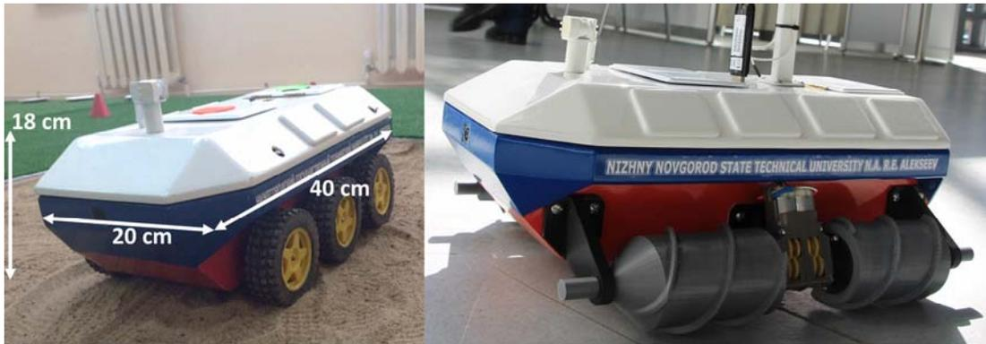
**Figure 10.** The model design and the laboratory robot.
