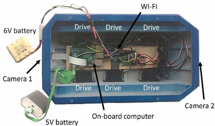
**Figure 12.** The robot modules structure.
