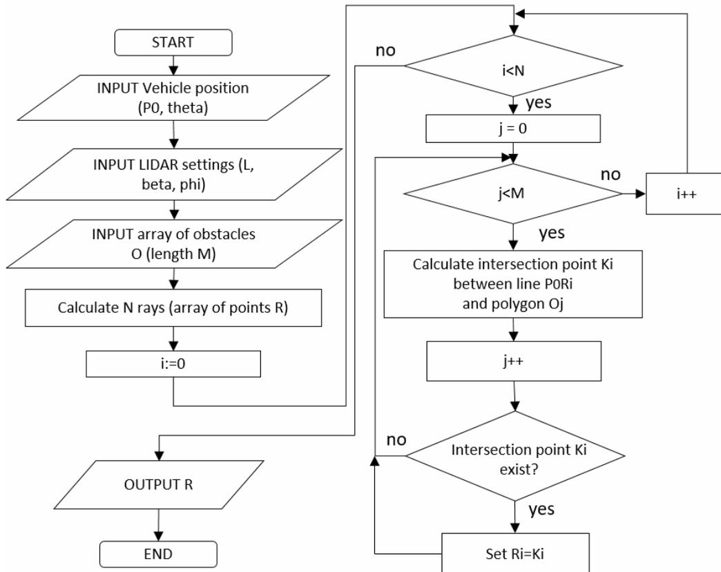
**Figure 7.** Virtual LIDAR operation flowchart.
