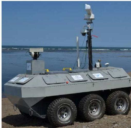
**Figure 1.** The mobile robotic system for coastal zone monitoring: wheels movers.
