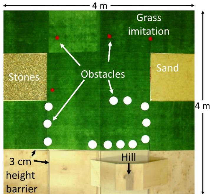
**Figure 15.** The laboratory environment for simulation of unmanned movement in coastal zones conditions
