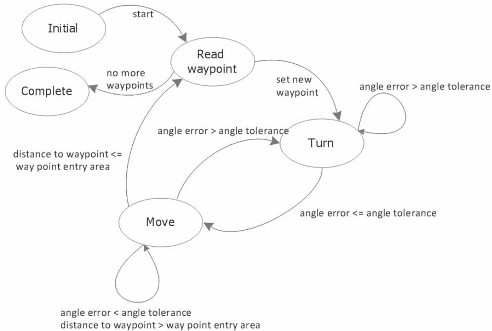
**Figure 8.** The robot controller model.
