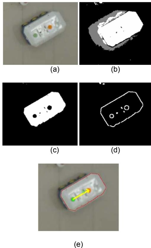
**Figure 9.** Stages of image processing: original image (a), background subtraction (b), noise filtering (c), contours detection (d), position and orientation detection (e).
