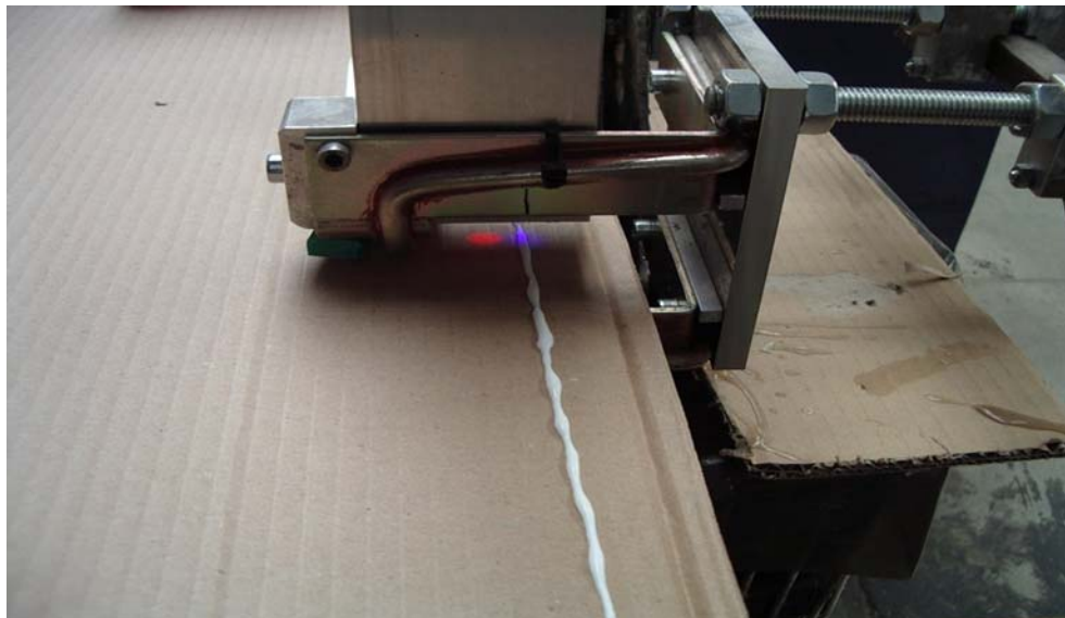
Figure 7. Detecting the presence of adhesive on corrugated paper.
