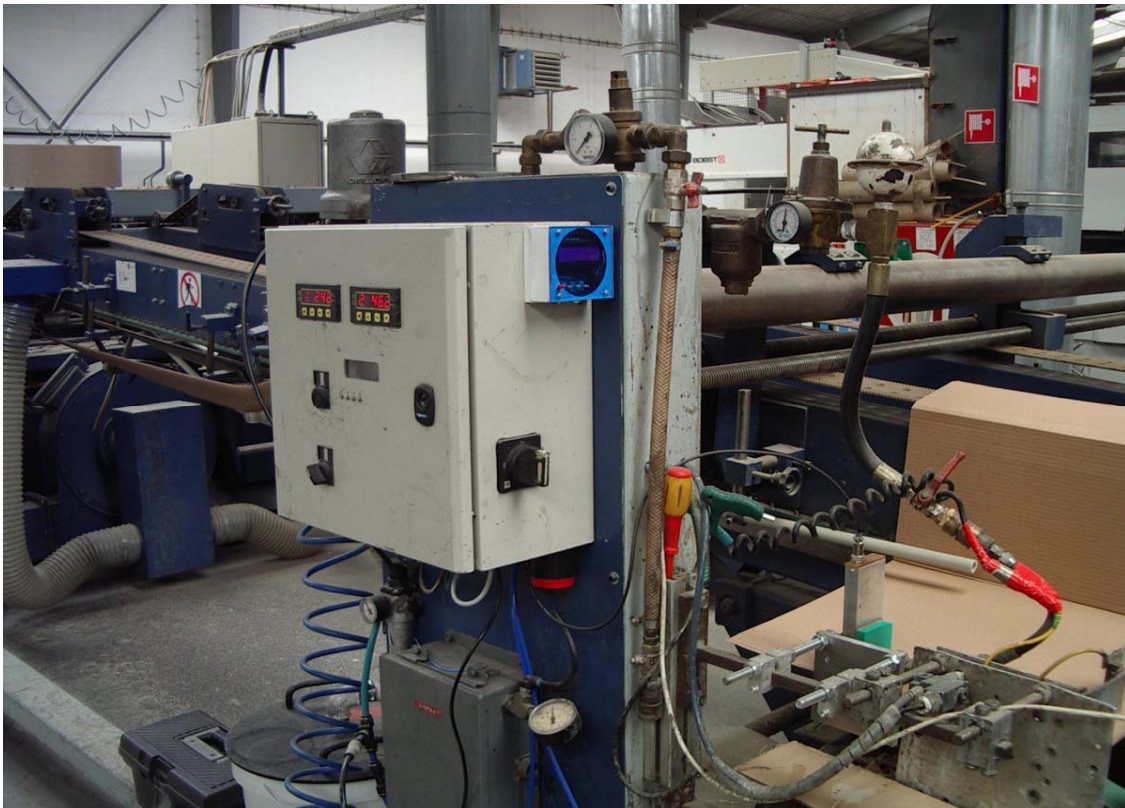
Figure 5. Practical realization of the device for checking the accuracy of application of the adhesive.
