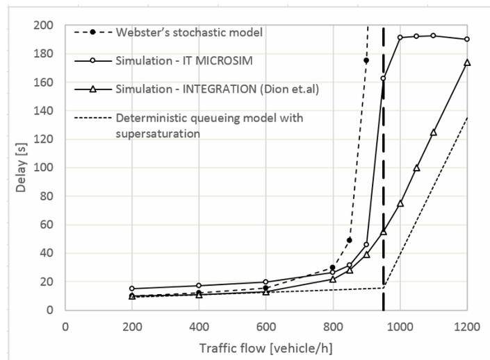
**Figure 3.** Comparison of models for delay times estimations.
