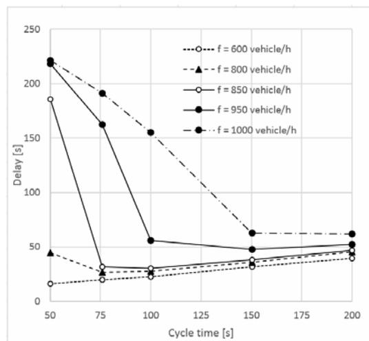
**Figure 4.** Average delay time in function of the traffic light cycle time.
