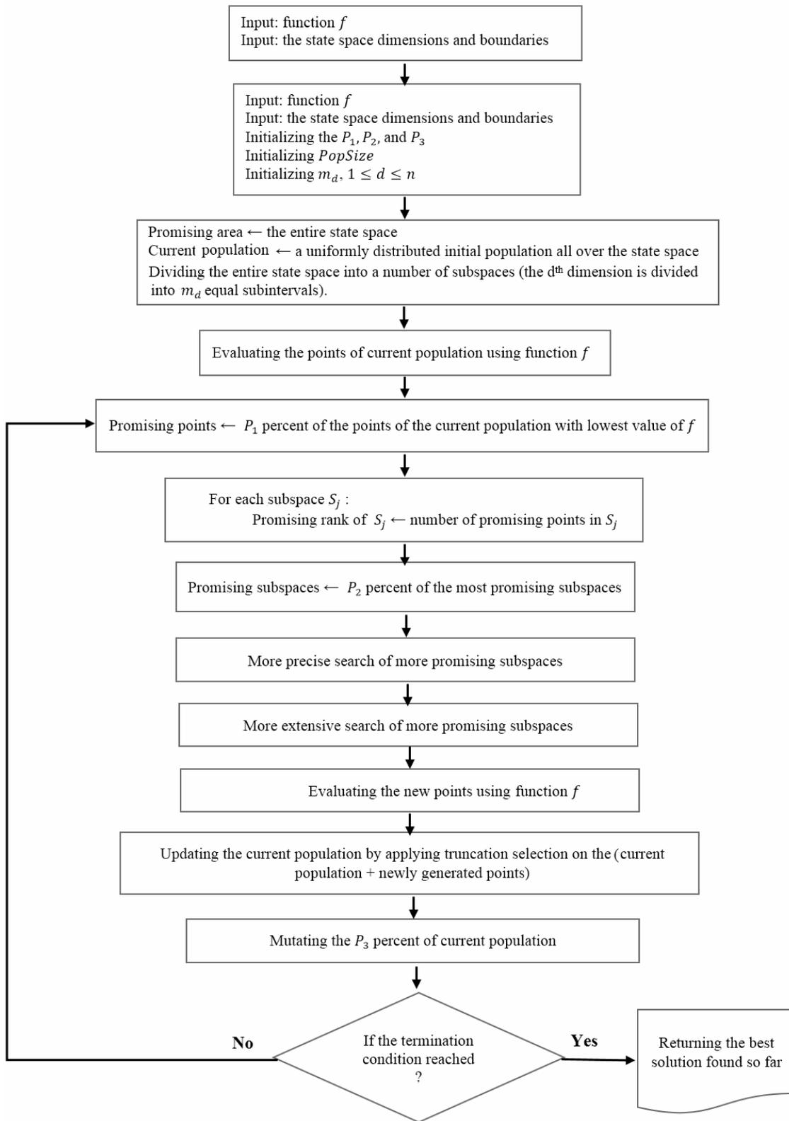
Figure 3. Flowchart of the fractal-based algorithm.
