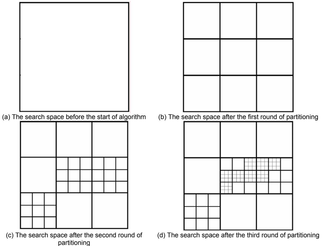
**Figure 2.** Forming the self-similar and fractal-shaped structures in the state space during the run of the fractal-based algorithm (promising subspaces are gradually divided into smaller subspaces so as to be searched more precisely and more extensively).
