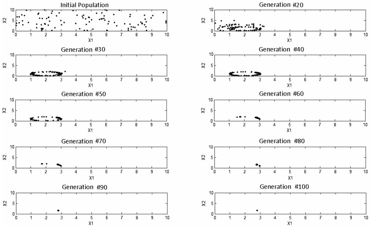
**Figure 9.** Distribution of candidate solutions during the run of the fractal-based algorithm for the Langermann function.
