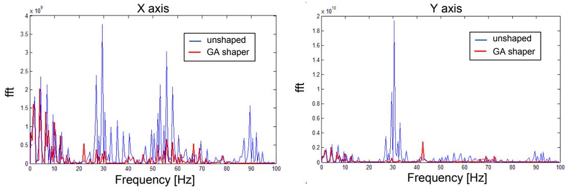
**Figure 10:** Power spectral density of unshaped and GA shaped square toolpath
