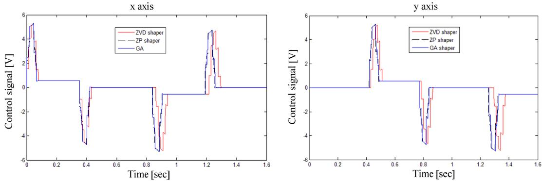
Figure 4: Control signal for axis drive in X and Y direction
