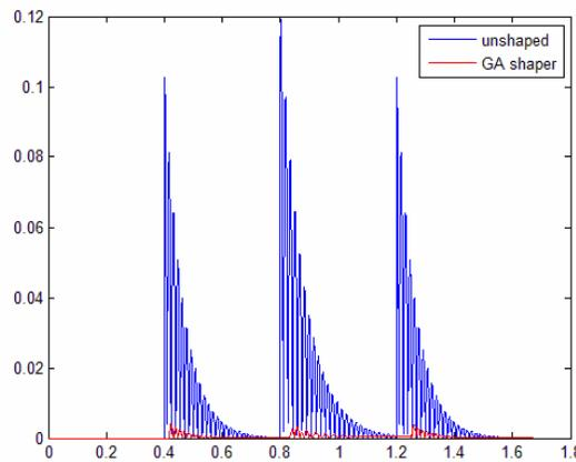
**Figure 6:** Contouring error response to unshaped and GA shaped position commands
