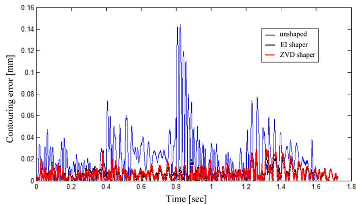
**Figure 8:** Contouring error response of the square to unshaped, EI and ZVD shaped positions
