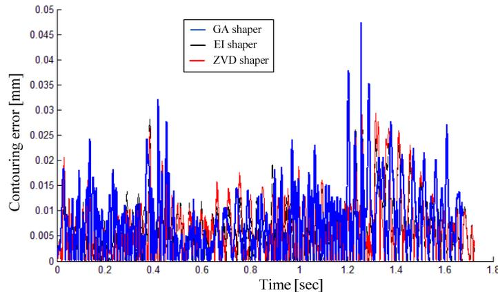
**Figure 9:** Contouring error response of the square toolpath to EI, ZVD and GA shaped positions
