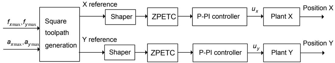
**Figure 3:** P-PI + ZPECT controller for axis feed drives
