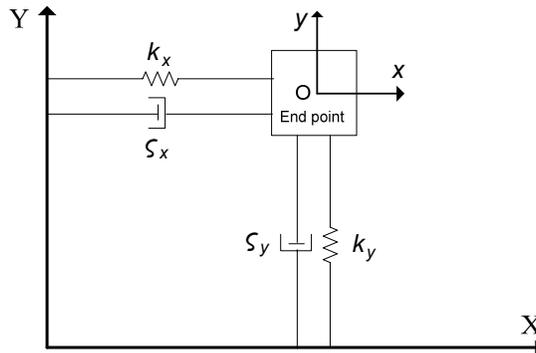
Figure 2: Biaxial model of CNC machine
