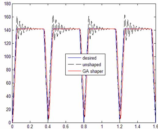
**Figure 5:** Feed response to unshaped and GA shaped position commands
