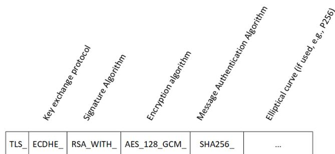
Figure 3. Structure of the cipher suite encoding
