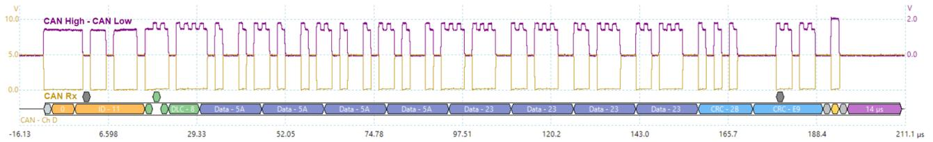
Fig. 12 Covert channel transmission at 1Mbps using the Aurix platform
