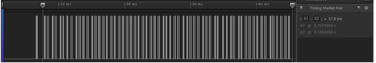
FIGURE 21. All 64 pairs of frames arriving on the bus during Time-triggered Minimax (capture with Salae logic analyzer).
