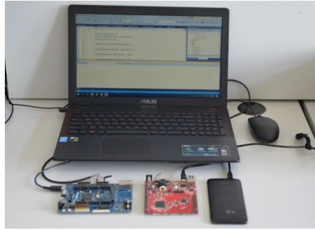
Fig. 4. Experimental setup: SAM V71, Infineon TC297 and an Android smartphone
