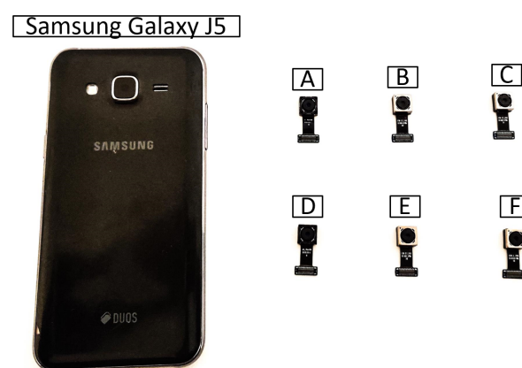
Figure 5. Samsung Galaxy J5 along with the six dismantled cameras.
