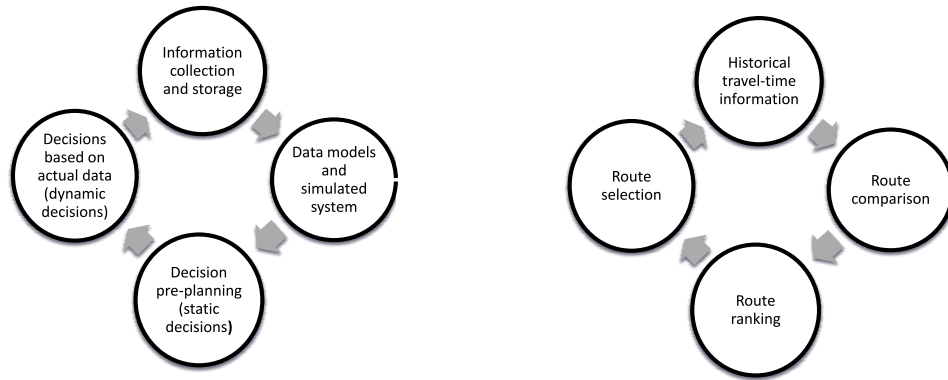
Figure 2: Generic four-stage decision loop of the agents (left) and its example for the routing problem (right)
