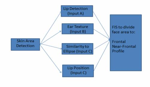
Figure 4. Block diagram of the proposed decision system
